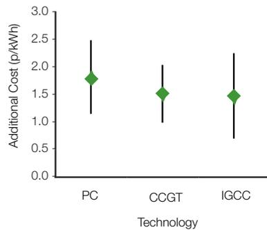
Figure 5: Additional Electricity cost depending on technology
